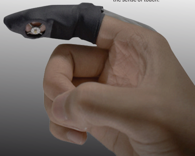
A device made from a new kind of artificial skin, shown covering a finger, simulates the sense of touch.
