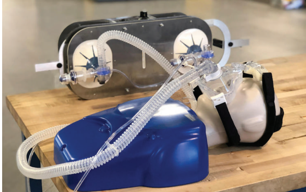
This low-cost ventilator was designed by a U.S.-British team. At its heart are breathing bags commonly carried on ambulances.
