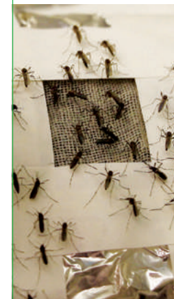
For five minutes, the researchers gave 100 mosquitoes access to a human arm. The insects did not bite when the arm was protected by dry graphene oxide (GO) film plus cheesecloth. With the cheesecloth only, there were plenty of itchy bites.
