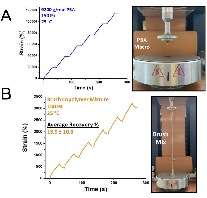
Creep Recovery experiment demonstrating the strength provided by an UHMW backbone: On its own, the polybutyl acrylate (A) shows no elastic recovery, while the brush copolymer mixture (B) shows an average elastic recovery of 16%. Images to the right provide a visual demonstration of the improved strength and elasticity of the material.
