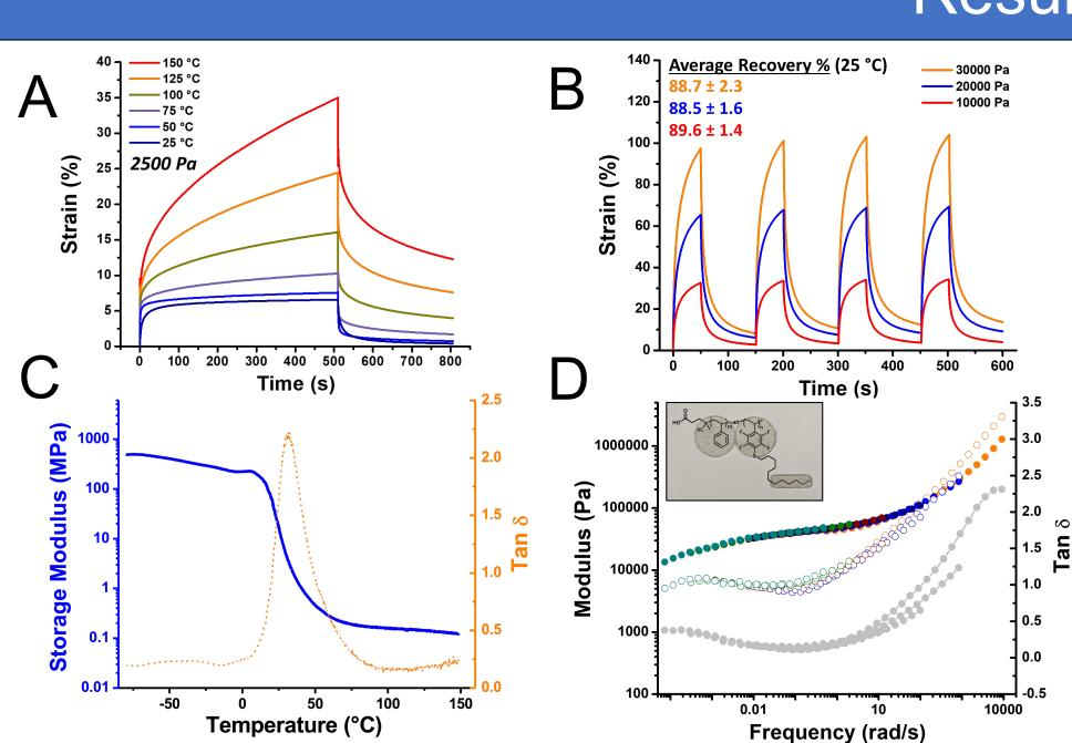
Rheological analysis of the dodecanethiol-functionalized polymer. (A) (B) demonstrate the polymer's elasticity, recovering nearly 90% of total deformation. (C) (D) show characteristics commonly seen in thermosets, such as (C) a continued rubbery plateau past 150 °C and (D) the storage modulus [closed circle] above the loss modulus [open circle], indicating network formation within the material caused by extreme amounts of entanglements at UHMW.
