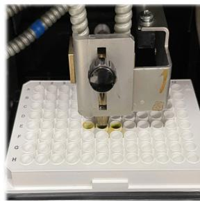
Figure 9: LSB50B well plate reader
