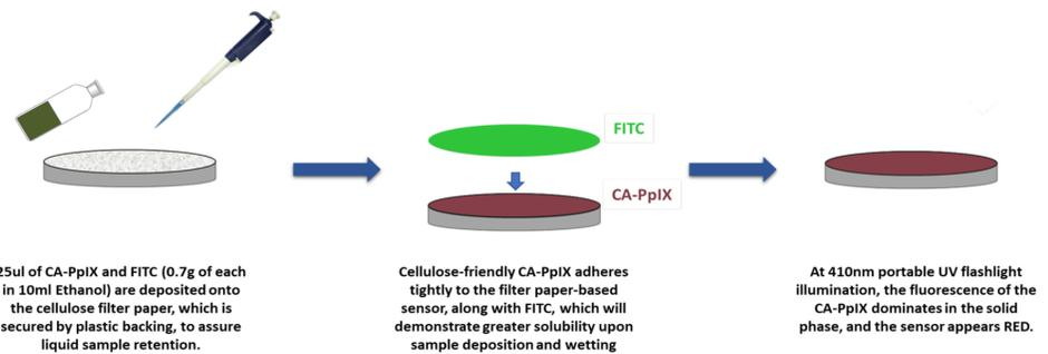
Fig. 11 (above): Construction of the DPH-Sensor
