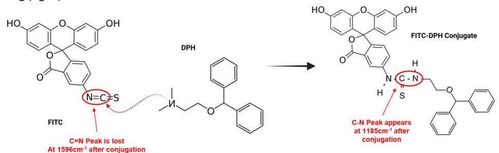
Fig. 7: Conjugation mechanism between the primary amine group of DPH, and the isothiocyanate group of FITC.
