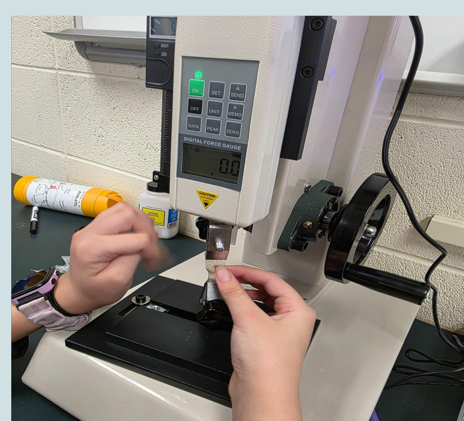
Testing bioplastic with digital pull force tester. (Photo taken by Linda Rost).
