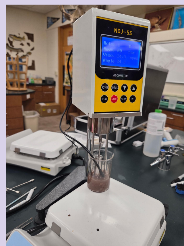
Testing viscosity of bioplastic using a viscometer. (Photo taken by Rye Rost).
