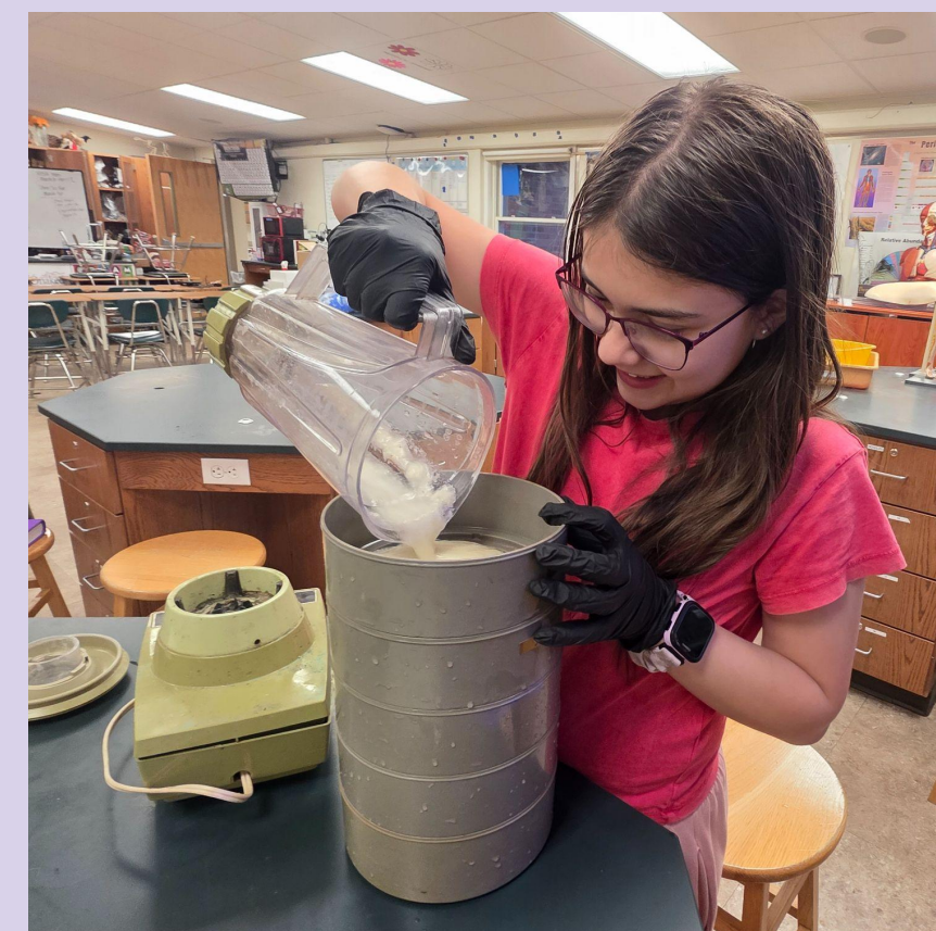
Sieving pulp-sodium bisulfite solution to 125 microns. (Photo taken by Linda Rost).
