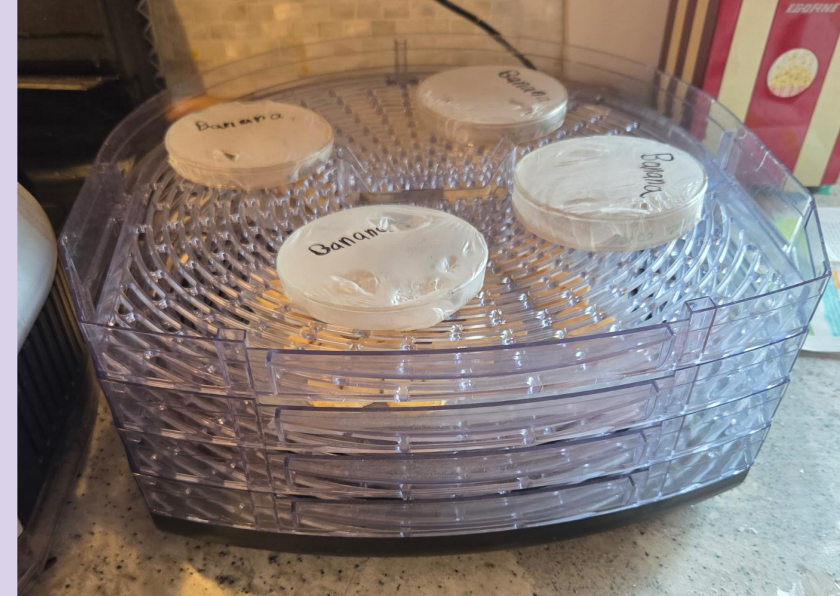
Drying bioplastic in dehydrator. (Photo taken by Rye Rost).
