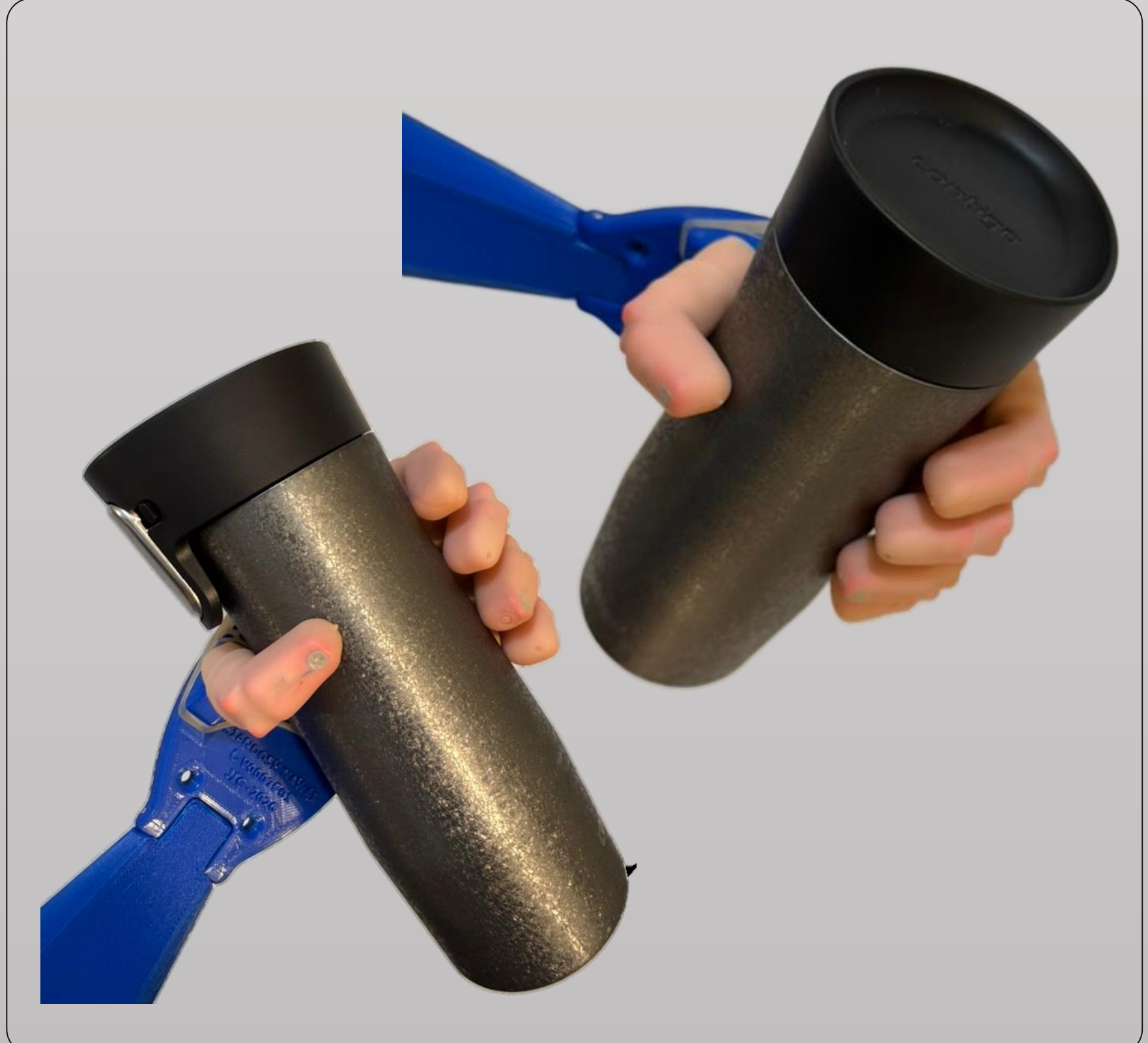
Prosthetic Hand 3D Print Prototype – 16 Fl-Oz Water Bottle–Grip test by Kianoosh Nawai
