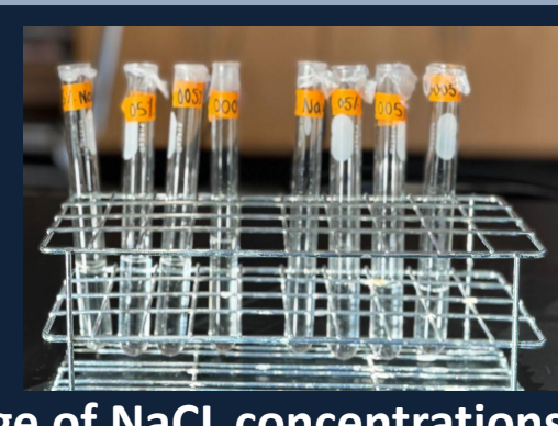
Image of NaCl concentrations after 1:2 Dilution: Images taken by Finalist using an iPhone 15, 2026
