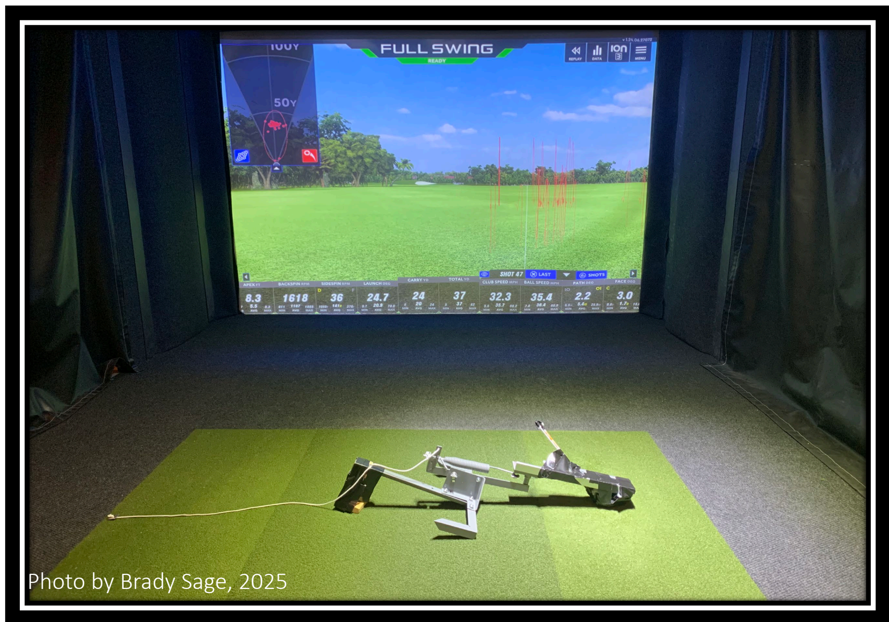
Modified clay pigeon shooter with driver head attached, positioned with simulator
