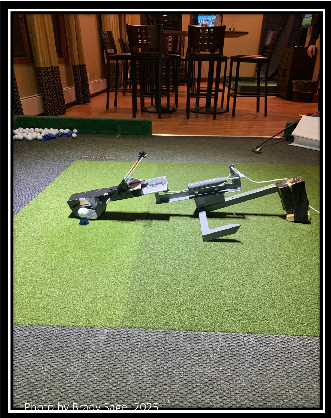
Modified clay pigeon shooter with driver head attached
