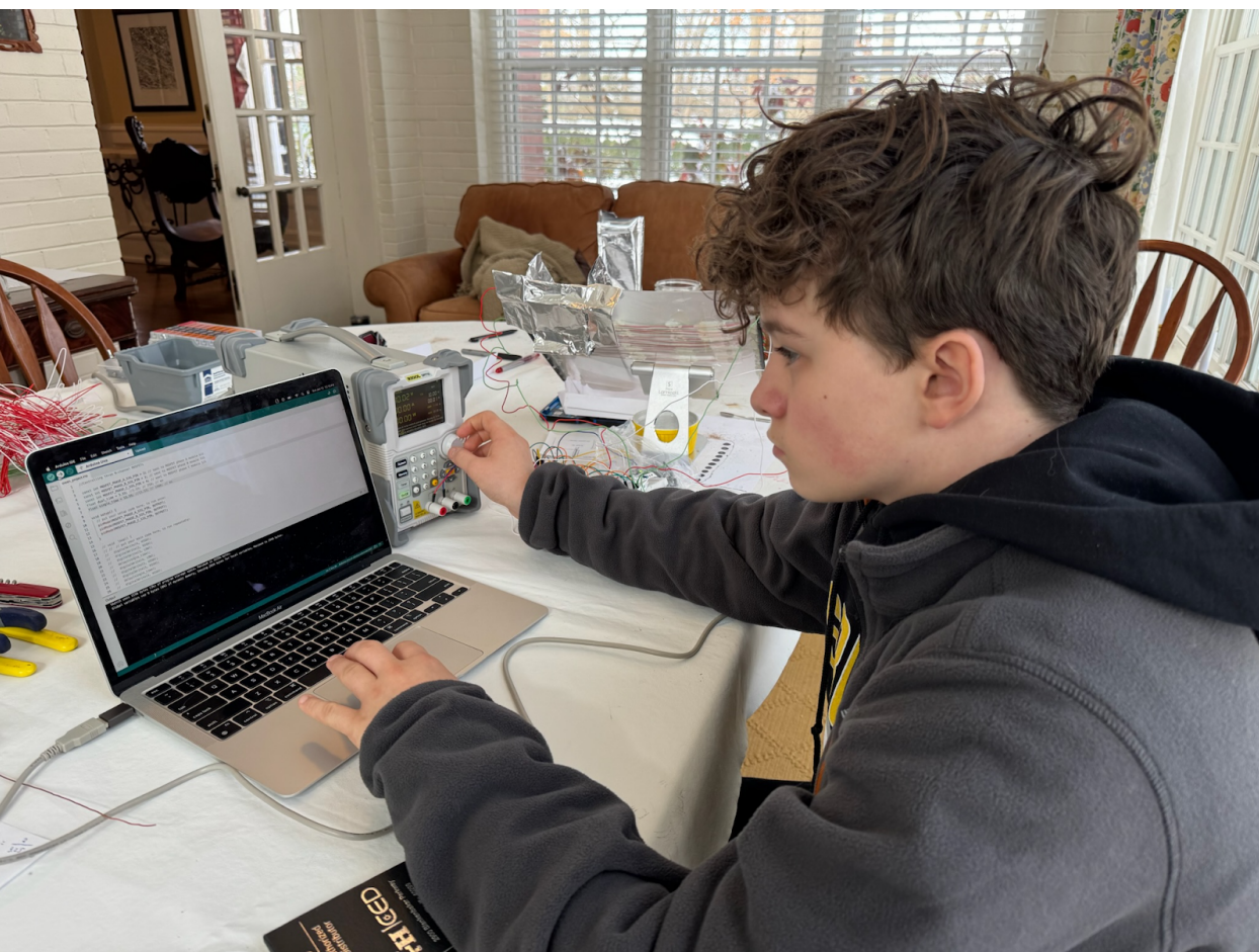
Pictured is the power supply being turned up to 10V and the code being run for the Arduino. Photo taken by guardian or student.
