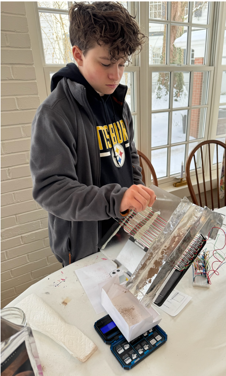
Pictured is the dropping of regolith onto the EDS in Earth's atmosphere. Photo taken by guardian or student.
