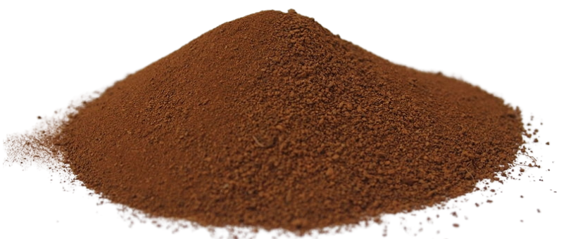
Let's Talk Science. (2025) A small pile of Martian regolith simulant JSC MARS-1A (Image). Let's Talk Science. https://letstalkscience.ca/educational-resources/backgrounders/soil-on-mars
