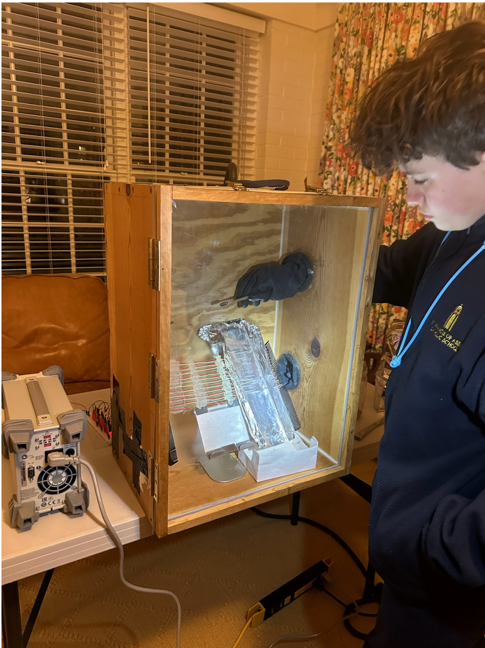
Pictured is the dropping of regolith onto the EDS in a simulated Martian atmosphere. Photo taken by guardian or student.
