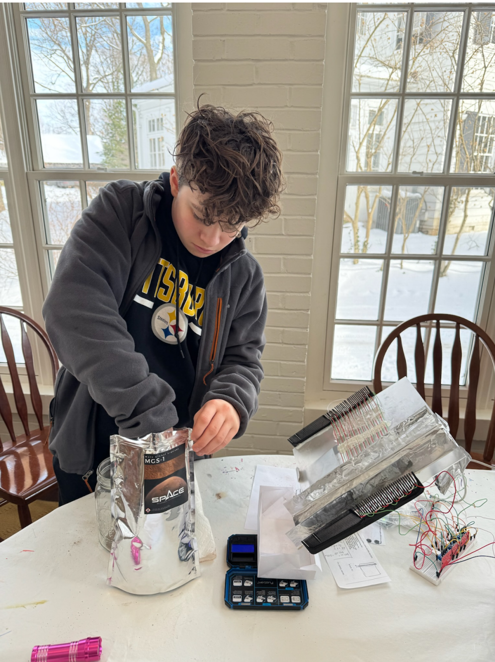
Pictured is the regolith being scooped in preparation for experimentation on the EDS with the box set on the scale. Photo taken by guardian or student.
