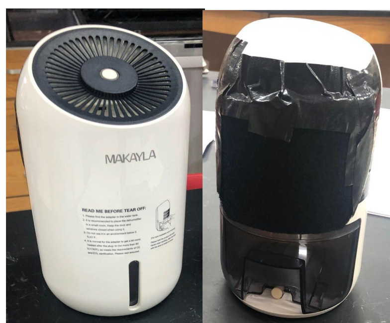
Figure 8a-b: Simple SHS Filtration was performed using a Makayla $20 portable dehumidifier (from Amazon), first on its on (left), and later with a $1 charcoal filter added (right).
