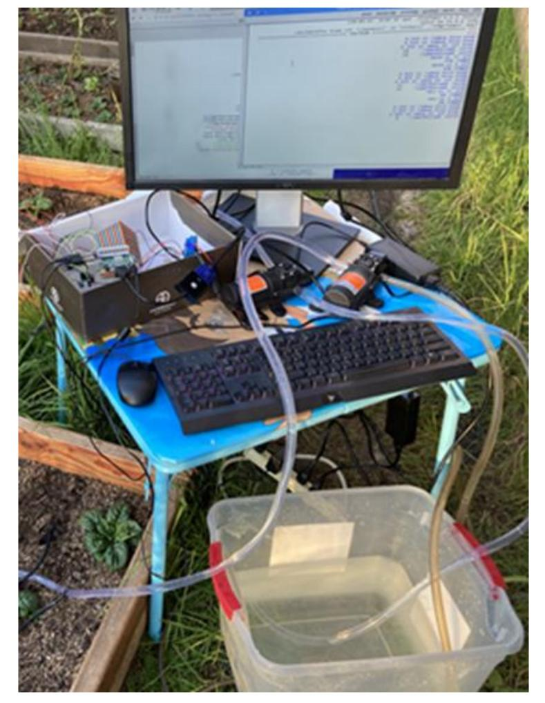
Figure 5: Irrigation control system with soil moisture sensor and pumps at the experiment plots
