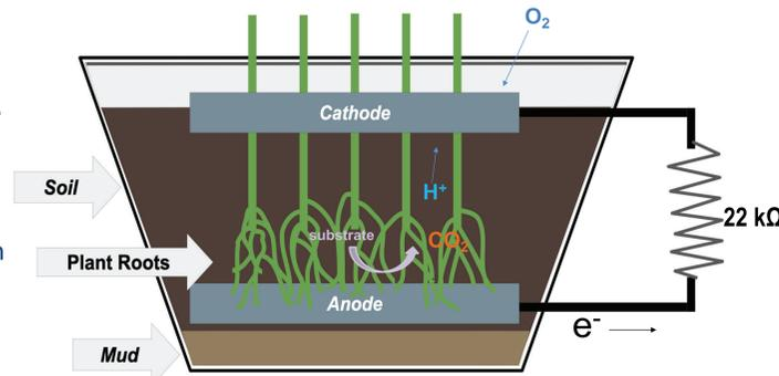
Example reaction at **anode** -- exoelectrogenic bacteria use organic compounds (e.g. sugars such as glucose) as substrate to produce electrons:
