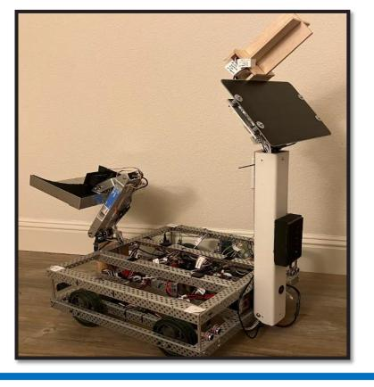
The engineering goal was to build an autonomous trashcollecting robot powered by the energy harvested from a high-efficiency suntracking solar panel.
